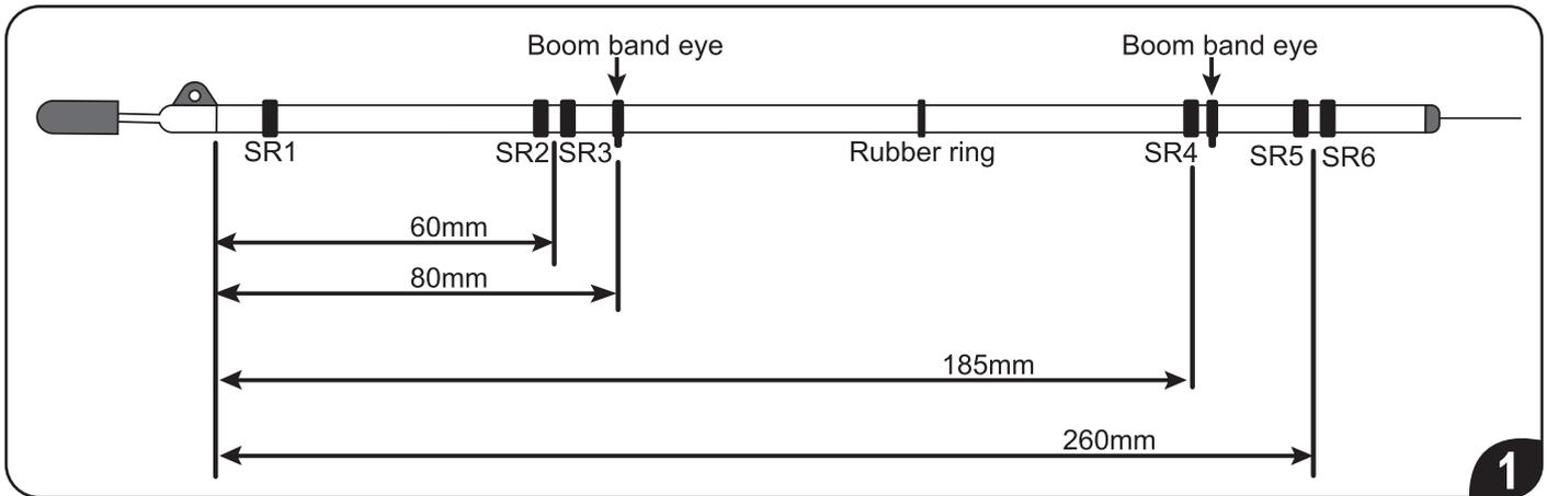
1. Adjust silicone rings ("SR" for short) positions on jib boom as shown.
