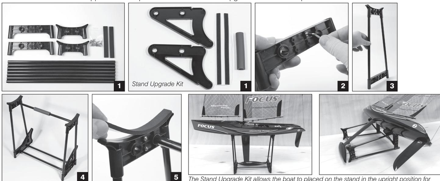
The Stand Upgrade Kit allows the boat to be placed on the stand in the upright position for easy access when rigging and indoor storage (shown above left), or the stand can be laid on its side and the boat secured in an almost horizontal position (shown above right) for additional stability outdoors.
