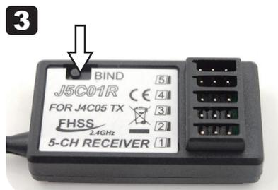
Note 1: You would also need to carry out the binding process if you were to replace the included receiver with another one.
