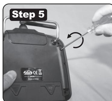
**NOTE:** If switch back form MODE 1 to MODE 2, firstly switch MODE button to MODE 2 under battery cover, screw off the left two screws, Screw down the right two screws, adjust down-left and up-right screws tightness so as to adjust the Throttle stick and Elevator stick spring tightness as you wanted.
