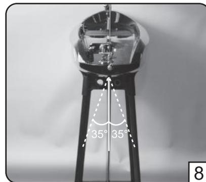
9. Rotate counterweight on front of jib boom by clockwise direction, adjust counterweight position, to make sure jib boom swing CG is located on SR2 and SR3 of Jib boom.
